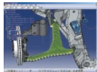
CATIA – Generative Part Structural Analysis 2 (GPS)
